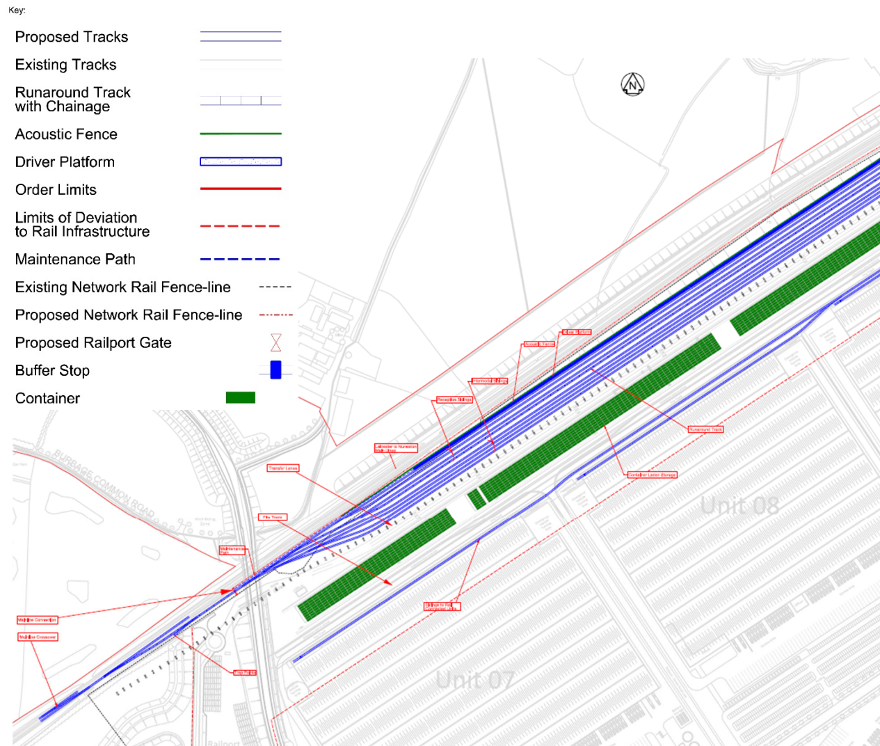
Fig 58. Western Arrangement of Main Reception sidings, intermodal sidings and container storage. Document Reference 2.25
